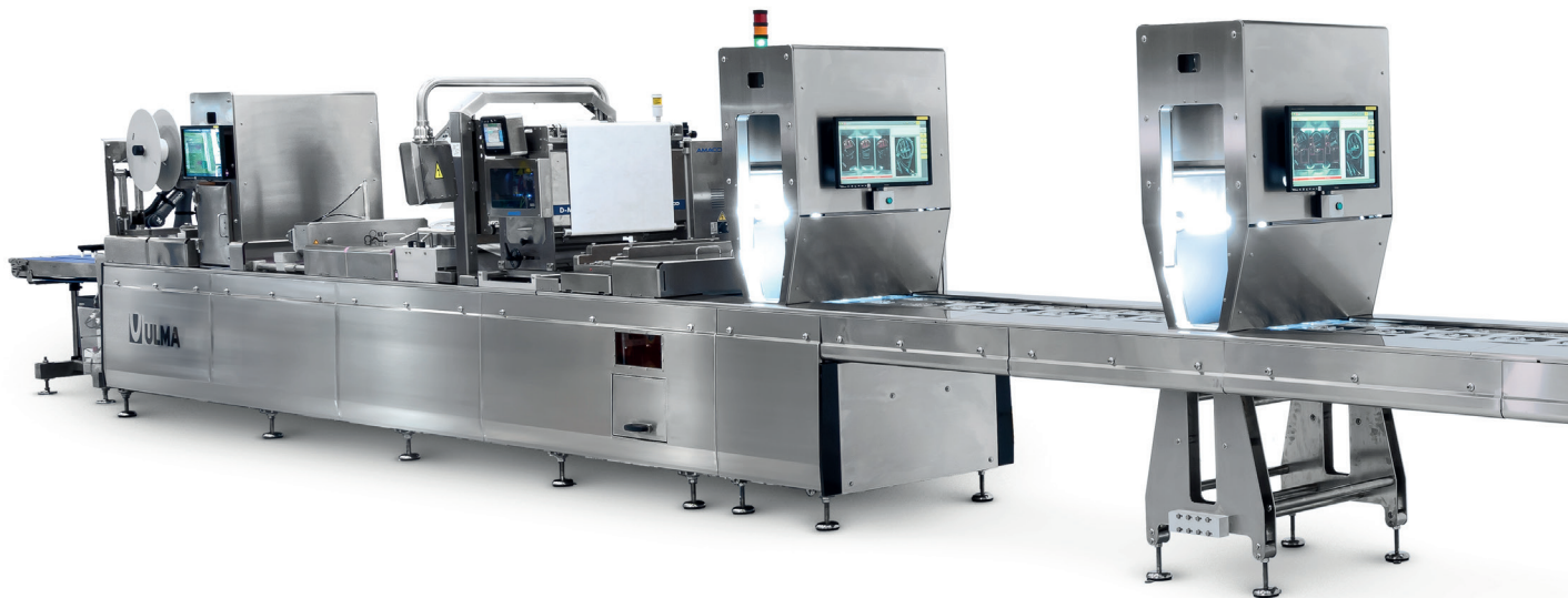
Catheter packaging line with vision inspection system and reject robot at the end of the line.
